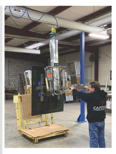
AL Systems provided a cost-effective labor saving solution that enables workers to easily pick up and move heavy components between workstations.
