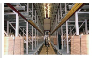
This system design allowed a larger amount of storage capacity from the building footprint. The single aisle for the S/RM added almost 1,000 more storage spaces.
