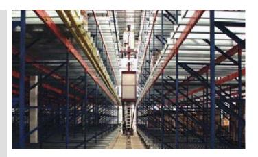
"At only 33' high, the facility's height is typical of conventional warehouses. But with our High Density AS/RS technology, its dense 4 level cubic storage requires a smaller building footprint, thereby having less impact on the environment around the facility." ~Dan Labell. President. Westfalia Tech.
