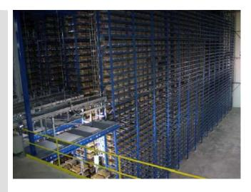
The new AS/RS provides high performance S/R machines with dual lateral belt transfer load handling devices that significantly increase the throughput per aisle
