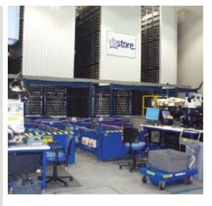
Quiet system operation was extremely important to the company. The system was designed so that at full operation, noise levels are less than 70db
