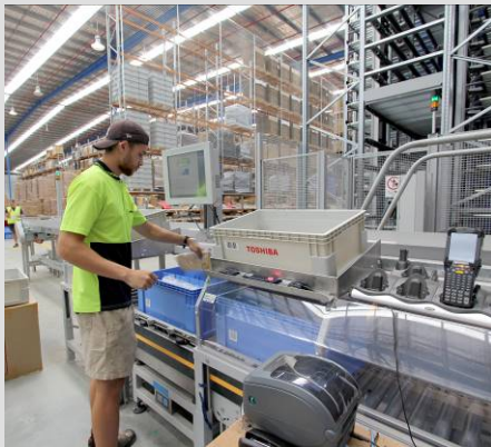
Inventory totes are delivered to the operator at the goods-to-person workstation.
