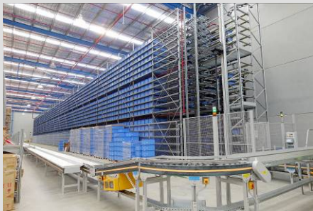
The goods-to-person piece pick system is a high density, compact solution that maximized the use of space in the warehouse.
