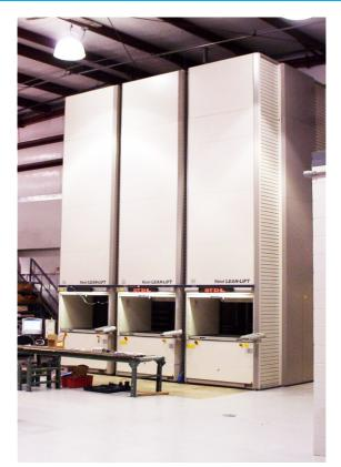
The lifts work together to cue the next part automatically so that the operator can move from lift to lift, minimizing any potential wait time for trays to be delivered to the access point. Totes and boxes are used to collect the various parts for each order, with a put-to-light system ensuring the right parts go into the right container. A pick-to-light system is used to pull fast moving items from bins nearby.
