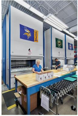
Thanks to digital compartment and sub-level indicators, even storage positions in very small configuration layout patterns can be identified easily. The combination of all these features ensures that orders are filled and shipped in record time – without errors.
