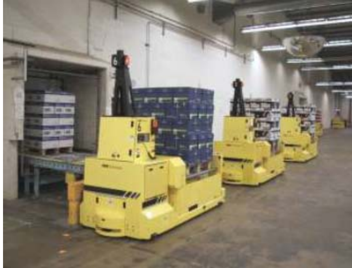
Linking packaging and palletizing lines is a common application for guided vehicles
