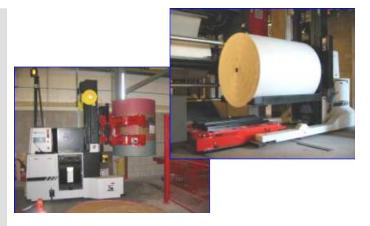
A fleet of 20 laser guided vehicles makes up a large component of the automated reel handling system at the Newspaper facility.
