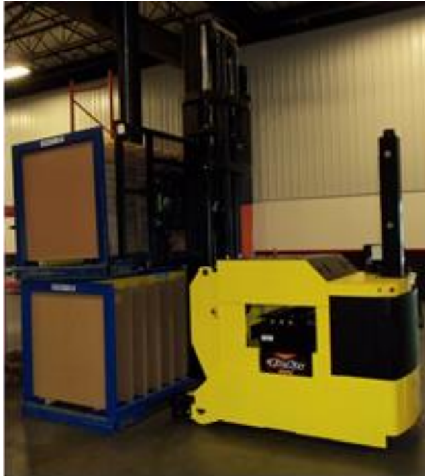
AGV transports Container and Underlayment Rolls on Pallets
