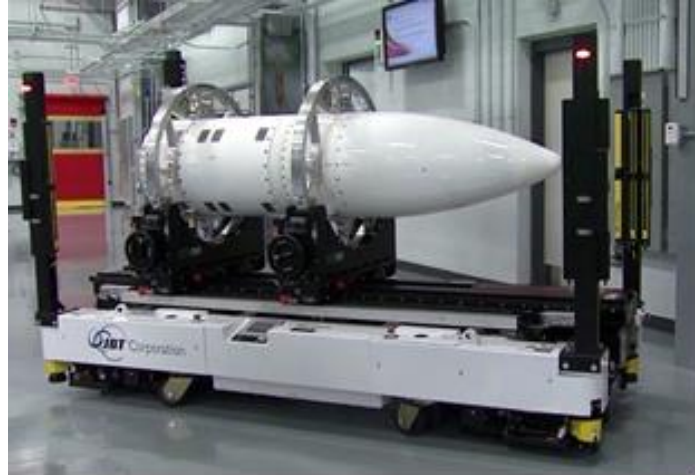
Laser-guided AGV system with hydraulic lift cylinders transport missiles through a factory
