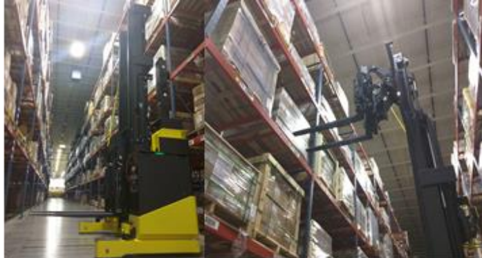
Outtrigger AGVs with hydraulic lift stacking pallets of an industrial manufacturing company
