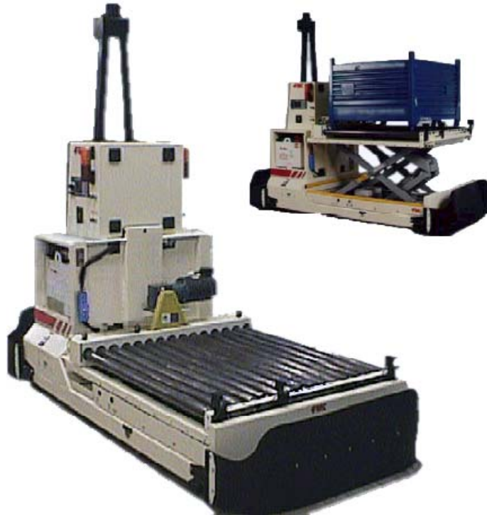
45 AGV Roller Deck and 6 AGV Scissor Lift Roller Decks service over 540 powered conveyors
