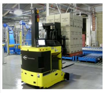
The dual fork carriage allows the AGVs to transport empty and full pallets simultaneously, eliminating the need for pallet dispensers at each packaging line.
