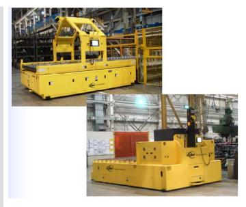
The AGVs are monitored in real time by the AGV Control Server to optimize material flow and allow the vehicles to share the same guide path.
