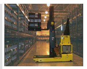
Seven dual stage lift mast Automatic Guided Vehicles (AGVs) deliver pallets of Oil Pans, Intake Manifolds, Exhaust Manifolds, Engine Heads and Engine Blocks in this engine manufacturing plant for a "Big Three" customer. The AGVs transport these materials from flow racks to intake conveyor positions.
