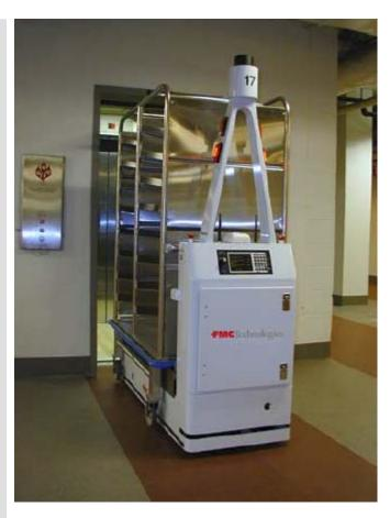
At this 11-story, 1,000+bed hospital complex, Automatic Guided Vehicles (AGVs) pickup and deliver materials on stainless steel carts to approximately 500 pick and drop off points. Each of the 43 vehicles can lift and transport loads weighing as much as 1,000 pounds throughout the facility.
