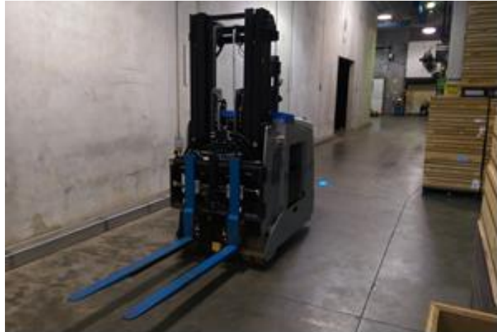
Forked Counterbalance AGV automatically moves and stacks pallets to/from WIP room & cooler
