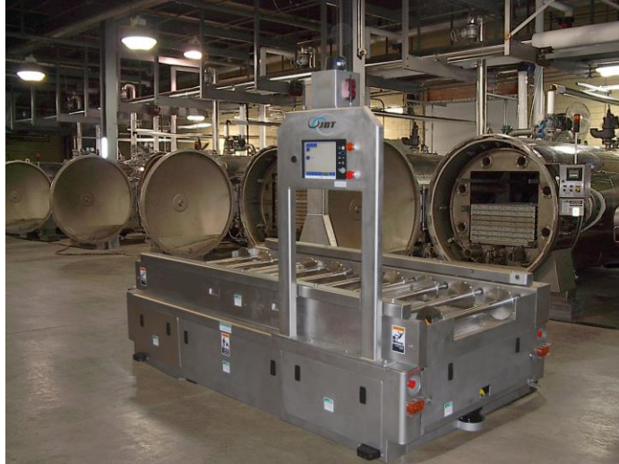
Unit Load AGV with Roller Conveyor Deck and "Pop-Up" Chain Conveyor/Stationary Rails -Attachment
