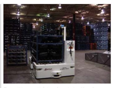
These vehicles use a side-fork transfer mechanism. All transfers are handled to the side of the AGV to facilitate increased material movement
