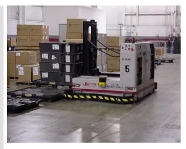
Theses vehicles use a side-fork transfer mechanism. All transfers are handled to the side of the AGV to facilitate increased material movement.
