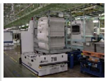
The vehicles handle most of the assembly parts from the incoming area to over 450 pickup and delivery locations at various stages throughout the manufacturing lines..
