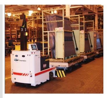
Tugger AGVs tow trailers which transport tractor chassis to/from manufacturing stations
